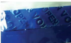
Result after being torn in ambient temperature
